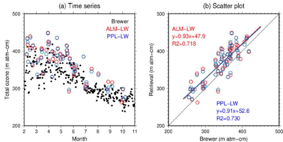
Figure 13. Seasonal changes (a) and scatter plots (b) for the total ozone of the ALM-LW (red), PPL-LW (blue), and Brewer spectrophotometer observations (black);  $y = ax + b$  and  $R^2$  are the linear fitting and coefficient of determination.
