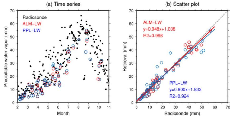
Figure 12. Seasonal changes (a) and scatter plots (b) for the precipitable water vapor of the ALM-LW (red), PPL-LW (blue), and radiosonde observations (black);  $y = ax + b$  and  $R^2$  are the linear fitting and coefficient of determination.
